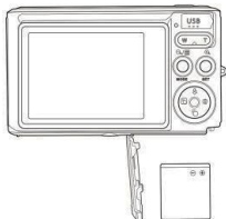
Install lithium battery
