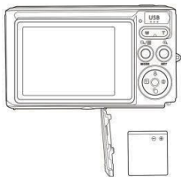
Install lithium battery
