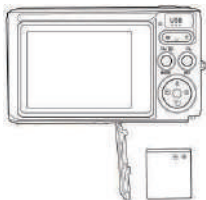
Install lithium battery
